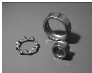
Outer ring, inner ring and cage halves are individually coated in a disassembled state
